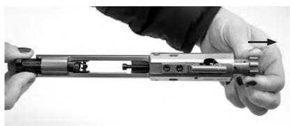
7 With the bolt pulled out, pull the firing pin straight back as far as it can go, until it stops.
