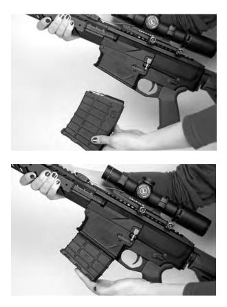
8 To chamber a round, pull back charging handle completely to the rear and let it go. Do not "ride" the charging handle. Let the rifle chamber the round. Any attempt to help or slow down the loading will result in the rifle jamming.
