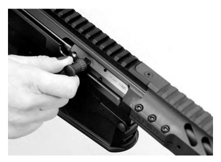
4 With the upper receiver assembly removed from the lower receiver assembly and with the side charging handle removed, pull bolt back and remove the bolt carrier group from the upper receiver assembly.
