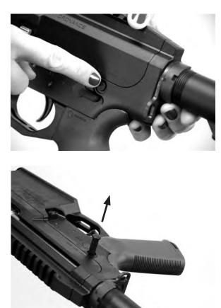
**3** Remove the charging handle by pulling it out firmly. Pull it straight out, away from the bolt carrier. The side charging handle is captured in the bolt carrier by a detent. It is held into place much like some semi-automatic shotguns.
