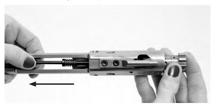
8 While holding the firing bin back, push bolt in and line up cam pin so that it can be removed. It must be able to clear the gas key.
