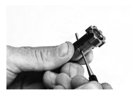
14 Clean out all of the carbon, brass and foreign debris from the extractor and on the inside of the bolt.
