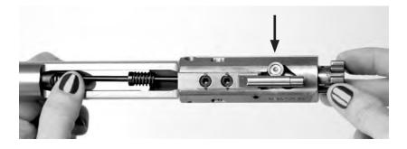
9 Remove the cam pin. Cam pin must be perfectly aligned in slot for removal.
