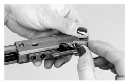
**10** After cam pin is removed, pull bolt out from the bolt carrier
