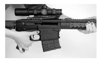
15 If your rifle experiences a jamb, place rifle on "SAFE". Remove magazine. Pull back charging handle and lock back with bolt catch. Clear rifle by removing cartridge. Replace magazine and re-charge rifle.
