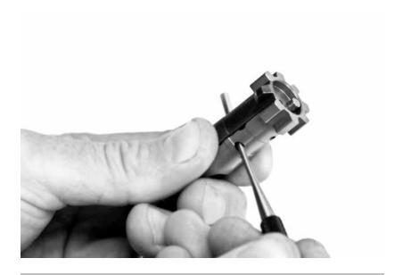
**14** Clean out all of the carbon, brass and foreign debris from the extractor and on the inside of the bolt.
