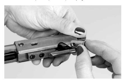
**10** After cam pin is removed, pull bolt out from the bolt carrier
