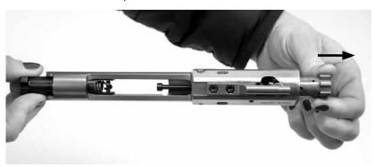
7 With the bolt pulled out, pull the firing pin straight back as far as it can go, until it stops.
