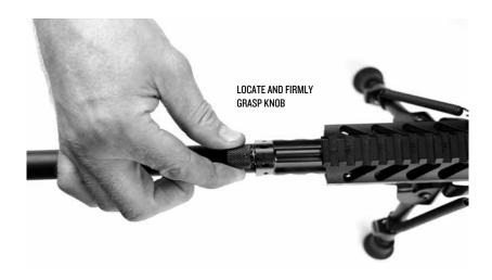
PUSH KNOB INTO GAS BLOCK AND ROTATE TO DESIRED SETTING. YOU CAN USE YOUR FINGERS, A 9/16 OPEN ENDED WRENCH, OR THE SIDE CHARGING HANDLE FOR MORE LEVERAGE.
