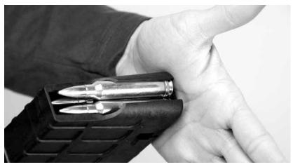
7 Insert magazine into rifle. Fully seat magazine by tapping the bottom. Pull down on magazine to insure magazine is captured by the magazine catch. A magazine can be inserted with or without the bolt open.
