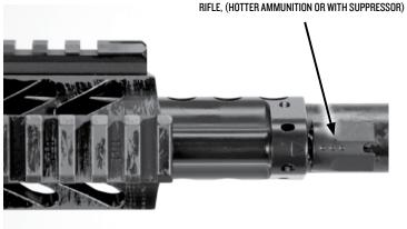
Having your setting on one or two dots should only be used if using a sound suppressor. The adjustable gas block does not have a setting to completely shut the gas off. Closing off the gas port from fully open (four dots) may cause your rifle to short stroke or not cycle.
