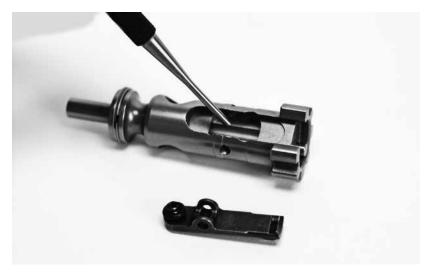
Your bolt carrier group is now completely field stripped for cleaning.
