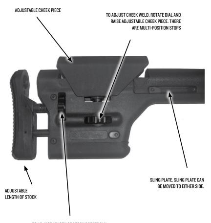
TO ADJUST LENGTH OF STOCK, ROTATE DIAL AND EXTEND STOCK BUTT PLATE. THERE ARE MULTI-POSITION STOPS
