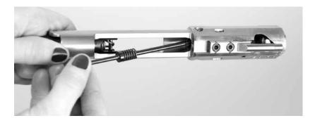
**12** Clean carbon from firing pin and spring. After cleaning, lightly lubricate spiring and firing pin with CLP.
