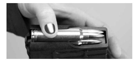
Ensure cartridges are seated at the back of the magazines by tapping the back of the mag.
