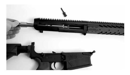
5 Use a punch or bullet tip to push firing pin retaining pin from the bolt carrier. Remove the firing pin retaining pin.
