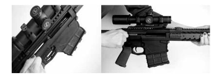
9 If the bolt is open, you can pull back on the charging handle to release the bolt or depress the bolt catch to release the bolt.
