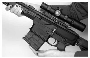
8 To chamber a round, pull back charging handle completely to the rear and let it go. Do not "ride" the charging handle. Let the rifle chamber the round. Any attempt to help or slow down the loading will result in the rifle jamming.
