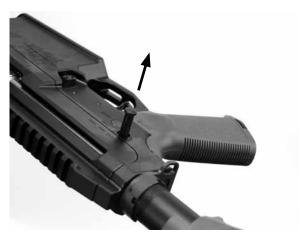
3 Remove the charging handle by pulling it out firmly. Pull it straight out, away from the bolt carrier. The side charging handle is captured in the bolt carrier by a detent. It is held into place much like some semi-automatic shotguns.
